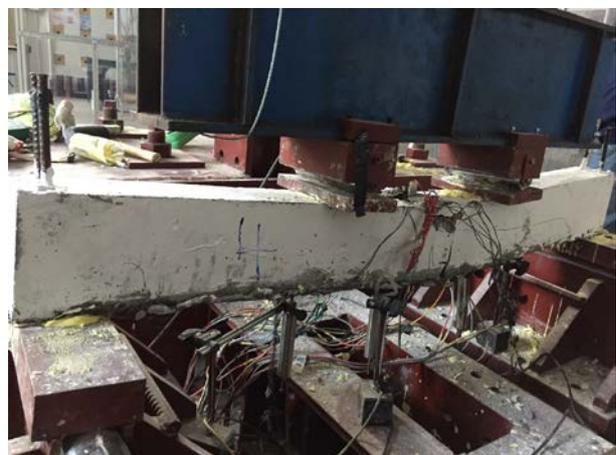
**Fig. 4.** Four-point bending test set-up
