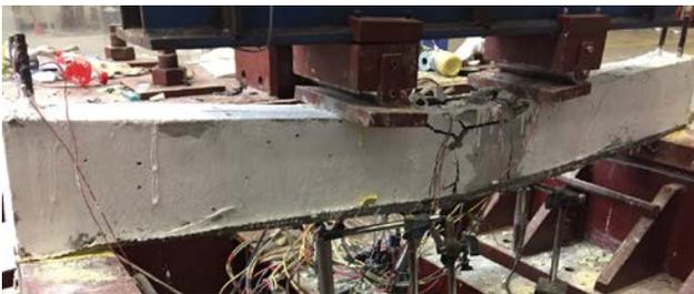
**Fig. 5.** Failure mode of tested beams
