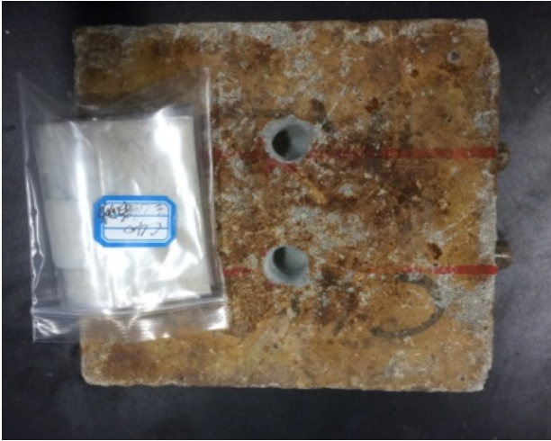
Fig. 6. Concrete block powder extraction
