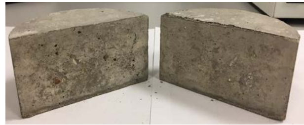
a) Control (flat surface): Interface debonding.
