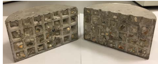
b) Pyramid (PY) texture: Interface debonding and fracturing of the concrete
