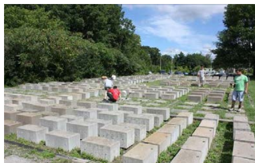
Fig. 1. Concrete blocks disposed on the CANMET outdoor exposure site
