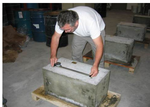
Fig. 3. Measurement on the longitudinal axis on the top of a concrete block (gage length is 500mm)
