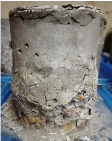
Fig. 10. Map cracking and detachment of a surface layer from silane treated concrete cylinders
