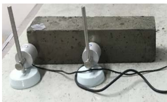
Fig. 2. Fundamental transverse frequency test
