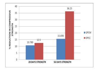
Fig. 5. Strength reduction due to NaCl attack on GPCM and OPCC
