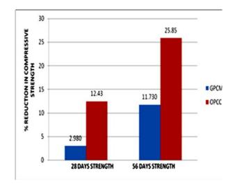
Fig. 3. Percentage of Strength reduction due to  $H_2SO_4$ Acid attack on GPCM & OPCC
