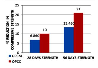
**Fig. 2.** Percentage of Strength reduction due to HCI Acid attack on GPCM and OPCC
