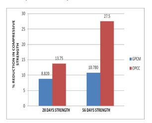
**Fig. 4.** Strength reduction due to Na2SO4 attack on GPCM and OPCC
