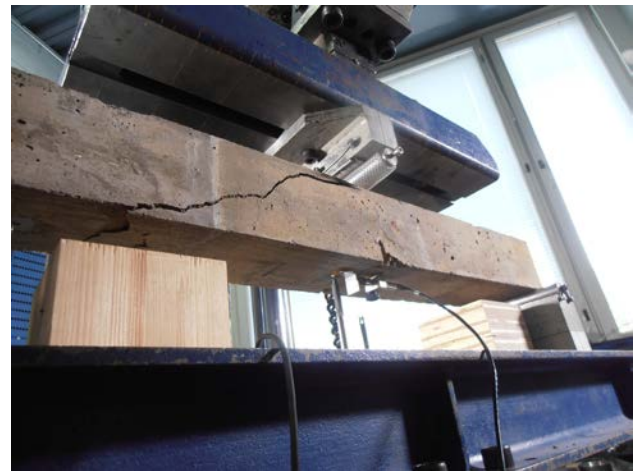
Fig. 3. Example of load-bearing capacity test by three-point bending: weldable hot-rolled ribbed steel bar, hot-dip galvanised (A8Zn-13), failure by shear
