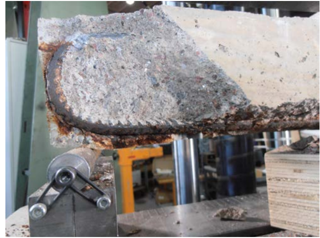
Fig. 8. Example of severe corroded beam after load-bearing capacity test by three-point bending: weldable hot-rolled ribbed steel bar (A12-22), failure by shear and anchorage
