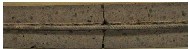
Fig. 10. Example of the opened beam specimen after load-bearing capacity test by three-point bending: cold-worked ribbed steel bar, hot-dip galvanised (B8Zn-29), failure by bending. Localised corrosion spots for instance at the crack (crack width w = 0.18 mm)
