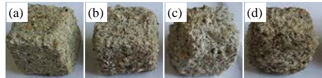
Fig. 9. Appearance of concrete specimens in sewage: a) CC1; b) CC2; c) CC3; d) CC4
