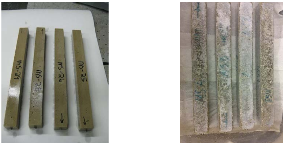
Fig. 3. Appearance of the mortar bars exposed to magnesium sulfate (MS): left – SC mortar bars after 18 months of exposure; right – OPC mortar bars after ~9 months of exposure.
