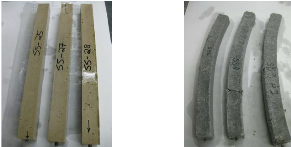
Fig. 2. Appearance of the mortar bars exposed to sodium sulfate (SS): left – SC mortar bars after 18 months of exposure; right – OPC mortar bars after ~9 months of exposure
