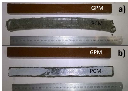
Fig. 2. Visual appearance of GPM and PCM samples after 52 weeks of exposure to 0.352 mol/L solutions of a) \text{Na}_2\text{SO}_4 and b) \text{MgSO}_4
