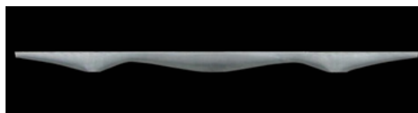
Figure 2.18: Concrete beam made with fabric formwork
