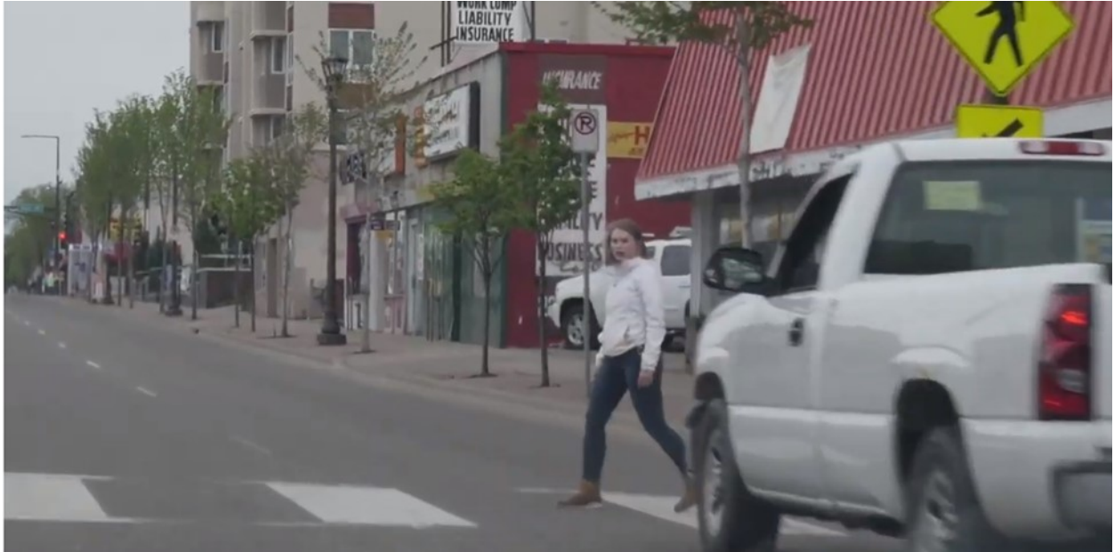
Figure 2.5 Still frame from Saint Paul PSA demonstrating short sight distances when driver stops near crosswalk
