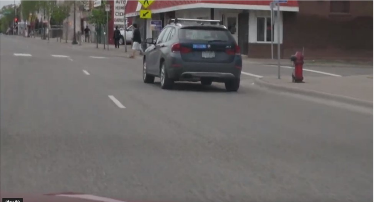
Figure 2.6 Still frame from Saint Paul PSA demonstrating long sight distances when driver stops far back from crosswalk
