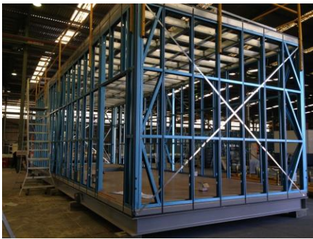
Figure 2: Light steel framework of a module Figure 3: High-rise modular building, Manchester, UK
