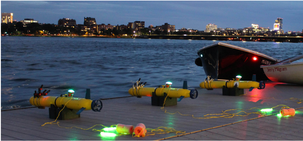
Figure 1.1: Our fleet of three low-cost, miniature commercial Bluefin SandShark autonomous underwater vehicles (AUVs) ready for deployment dockside at the Massachusetts Institute of Technology (MIT) Sailing Pavilion. They are named Platypus , Quokka and Wombat .
