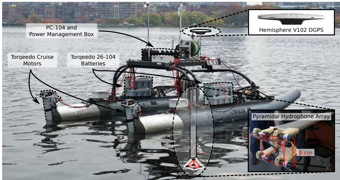
Figure 5.1: WAM-V autonomous surface vehicle outfitted with the piUSBL payload – the twin pontoon platform is equipped with differential drive Torqeedo Cruise motors powered by four Torqeedo 26-104 batteries, and navigates solely using differential GPS; it is outfitted with our piUSBL system with an 8cm pyramidal hydrophone array mounted on a submerged boom rigidly affixed to the port-side pontoon.
