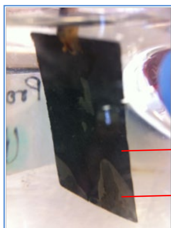
Figure 5.6: Illustration of the loss of polymerised layer/biofilm seen in all MFCs after 1 month of operation.
