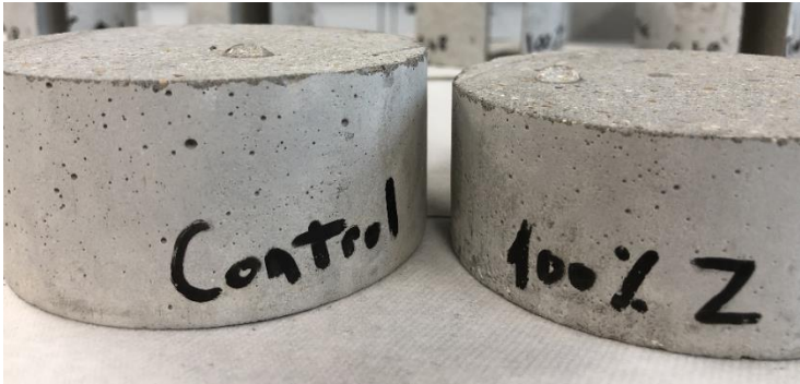
Figure 13: Drop of water at the surface of two specimens at t = 0mins
