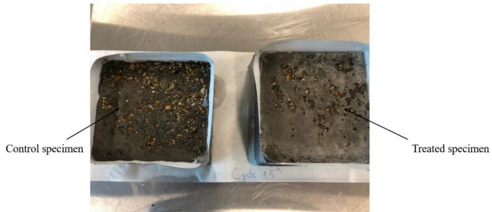
Figure 24: Results for the mix with river gravel after 15 cycles
