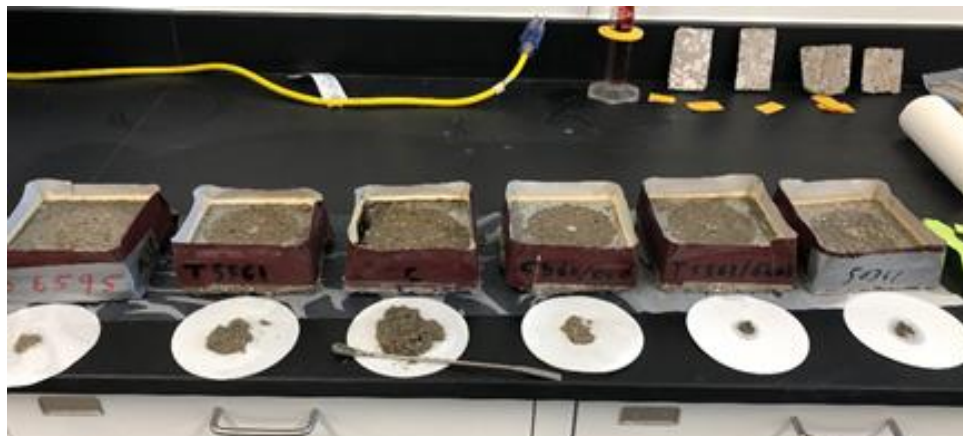
Figure 31: Visual assessment of Freeze/thaw damage and mass loss collection
