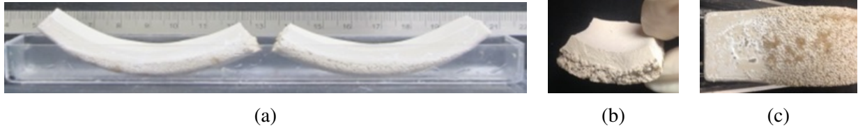
Figure 4.22: Pictures of the 80/20 kaolinite/sand mixture at the end of the drying test: (a) lateral photo showing the curled and broken sample; (b) front image of the broken section sample showing the soil segregation, with the larger sand grains settle at the bottom of the sample; (c) image of the bottom of the sample showing the deposition of the sand particles.
