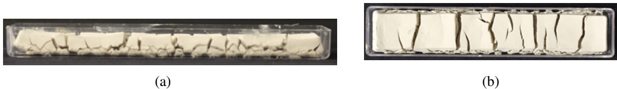
Figure 4.23: Crack pattern of the soil sample, 85% kaolinite with 15% silica sand at the end of the test: (a) side view; (b) top view
