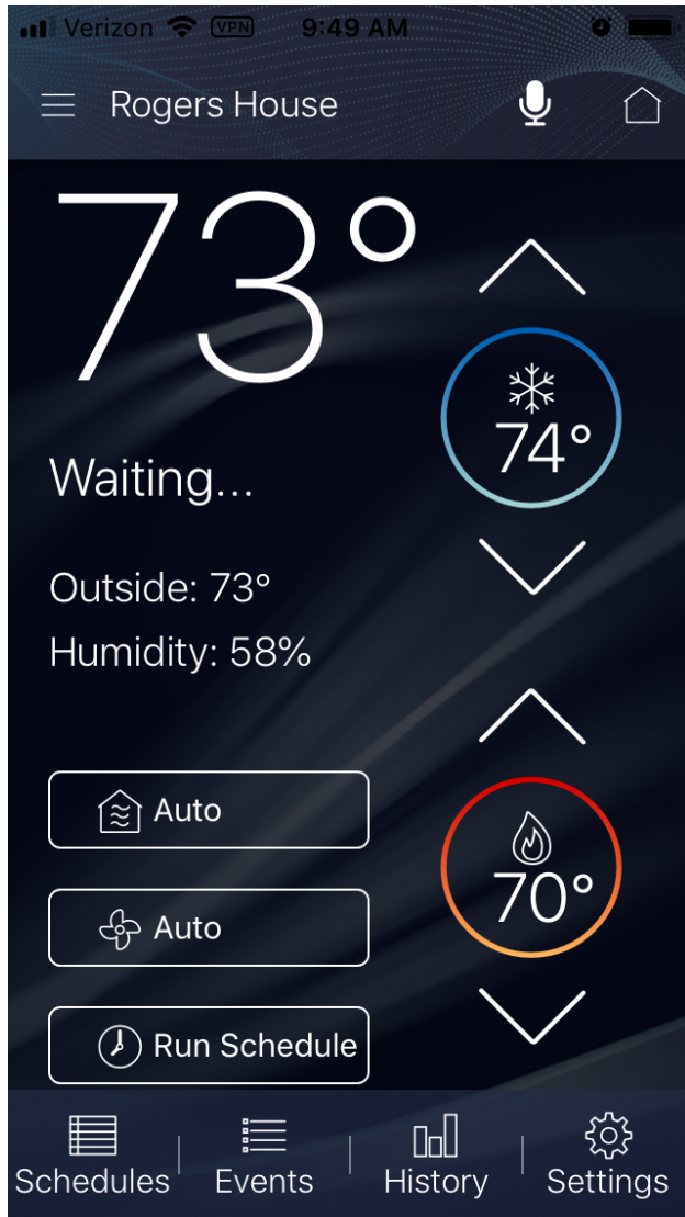
Figure A.8: A screenshot of the iOS mobile application that accompanies the Trane XL824 connected thermostat.
