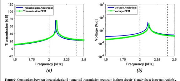
**Figure 3.** Comparison between the analytical and numerical transmission spectrum in short circuit (a) and voltage in open circuit (b). Dashed lines show the design trapping frequency range for the harvester.
