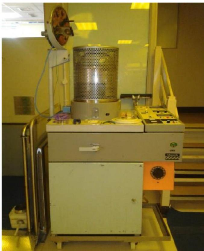
**Figure 4-12: Optical image of Edwards 306 thermal evaporator.**
