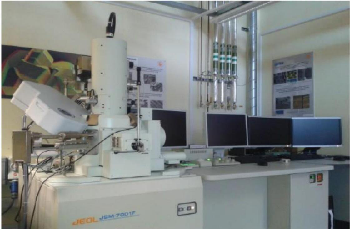
**Figure 4-6: Optical image of JEOL JSM-7001F field enhanced SEM.**
