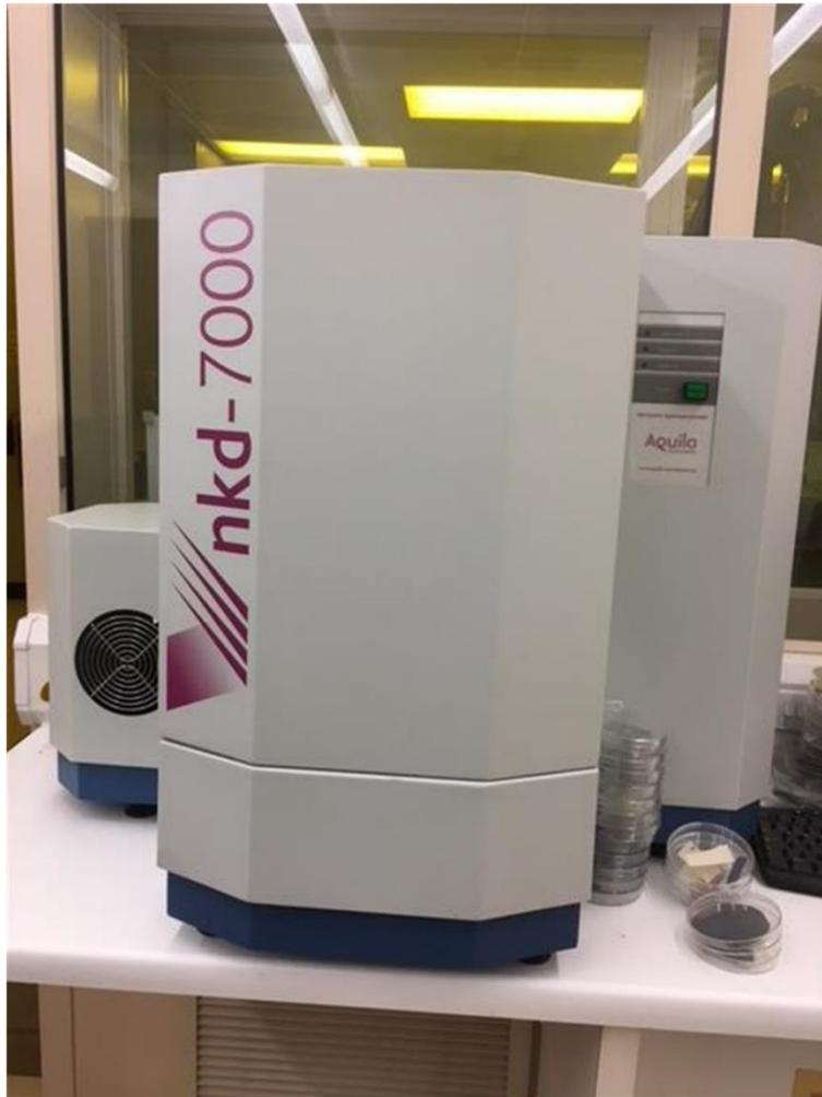
**Figure 4-5: Optical image of Nkd-7000 spectrophotometer.**
