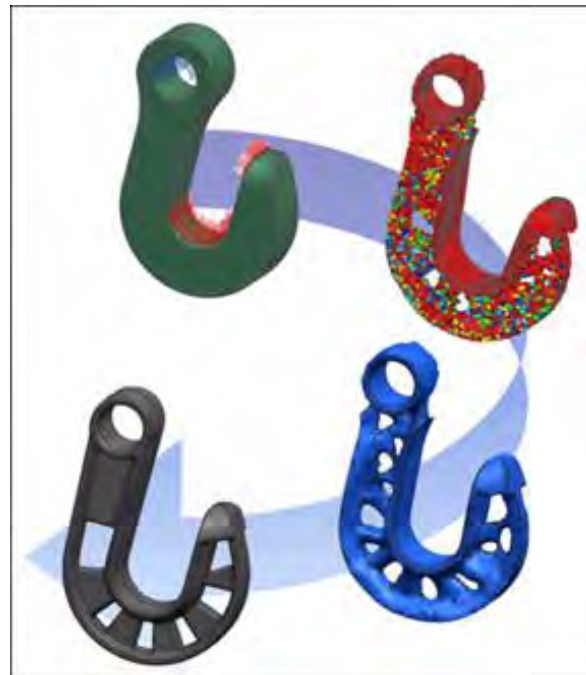
Figure 4.3 - Topology optimisation of a crane hook using NX8 [source: 35]
