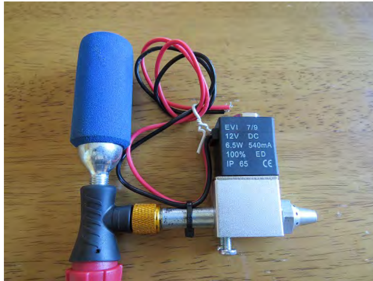
Figure 4.5: Complete air delivery system construction.
