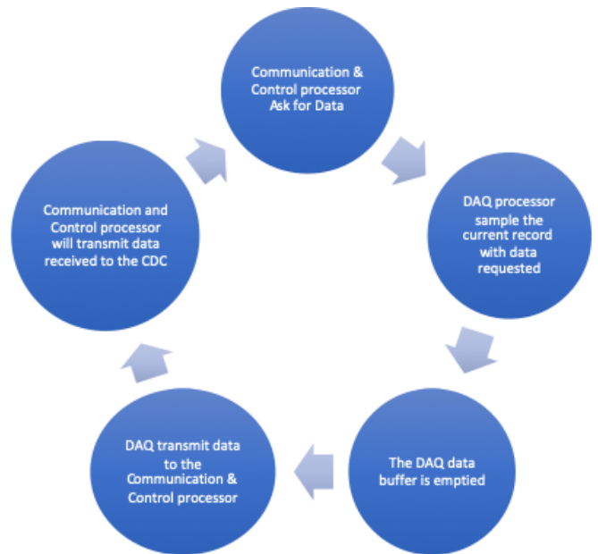
Fig. 6. Work-flow diagram for a data transaction between Communication & Control processor and the DAQ processor
