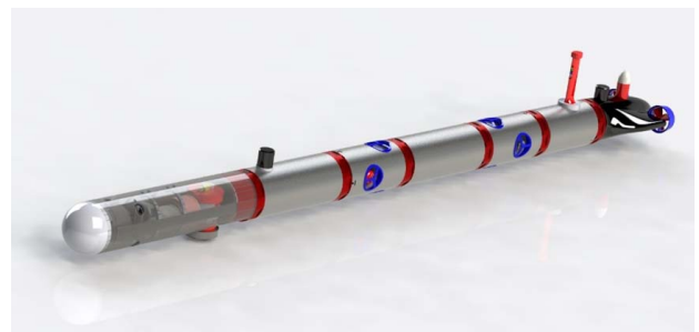
Fig. 1. Final CAD design of MARTA modular AUV
