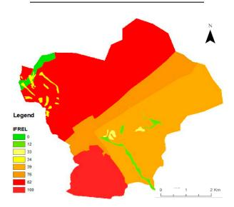
Figure 7. Relative Landslide Susceptibility Index (IF<sub>rel,j</sub>) for each lithology class.
