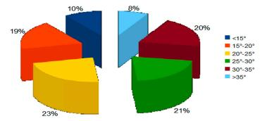
**Figure 9.** Instability processes occurrence (%) as a function of dip-slope classes, reported as different dip-slope ranges, represented with different colors.
