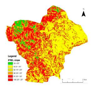
Figure 10. Map of the Relative Landslide Susceptibility Index (LSI<sub>rel,i</sub>) in front of the 'dip-slope' factor.
