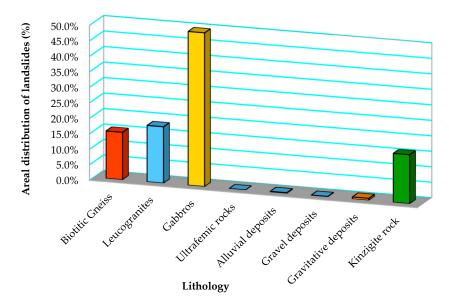
**Figure 5.** Areal distribution of landslides (%) in relation to the lithological substrate or bedrock (lithology).
