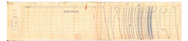
**Figure 2.** Original rainfall track recorded at Coggiola meteorological station. The maximum peak was recorded around 9 pm, with a rainfall amount 30 mm recorded in 30 min. The pluviogram has a rainfall amount resolution of 0.2 mm. The interval, from the bottom to the top of the pluviogram covers a span of 10 mm. The time resolution, reported on the horizontal axis, has a resolution of 1 h.
