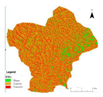
Figure 8. Relative Landslide Susceptibility Index (LSI<sub>rel,i</sub>) for each morphology class.
