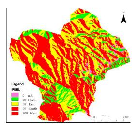
**Figure 11.** Relative Landslide Susceptibility Index ( $LSI_{rel,j}$ ) as a function of the aspect factor (n.d. is used in the map for the areas where the aspect is not definable, due to the poor level of detail of the available raster)
