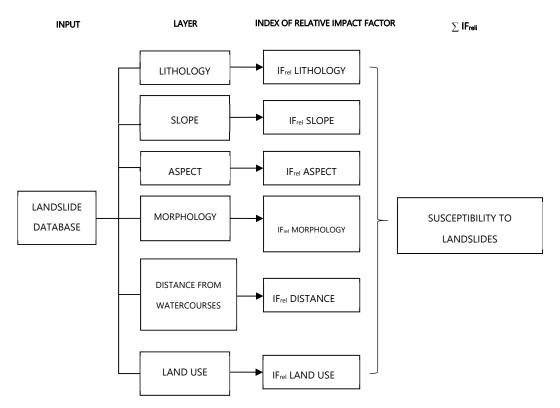
Figure 4. Flowchart of analysis for evaluation of the final impact factor (IF<sub>rel</sub>).
