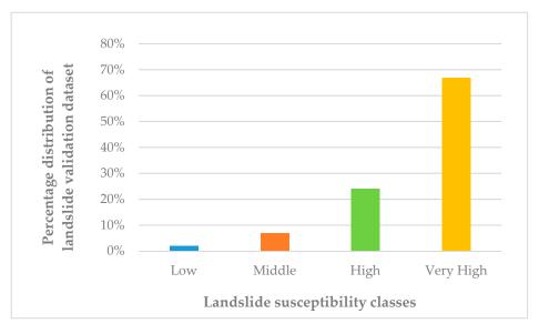
**Figure 15.** Results of validation process, using 1994 and 2000 landslides as the validation dataset. The majority of observed landslides fell within the 'Very High' (67%) or 'High' (24%) susceptibility classes.
