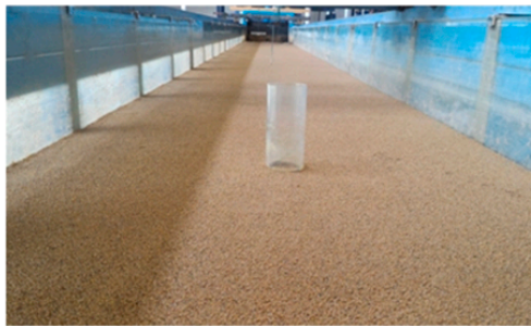
Snapshot after bed preparation and installation of pier
