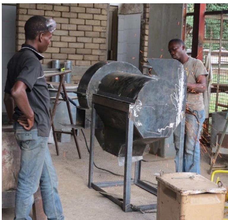
Figure 5. Training on assembling the multiple crop threshing machine.
