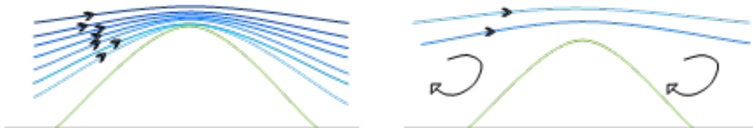
Figure 3.6: WASP estimation of flow over steep inclines (left) and real wind flow separation (right) [5]
