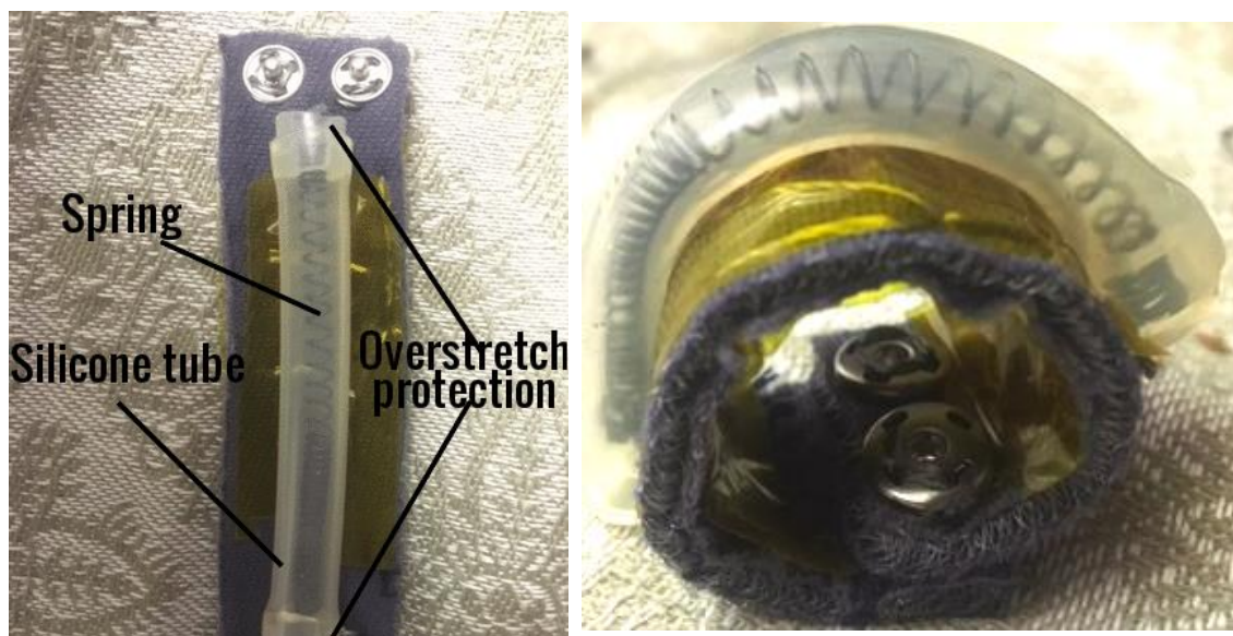
Figure 36: Final bracelet prototype stretched (left) and wrapped (right). Modifications regarding thermal insulation were adopted and inspired by the second prototype.
