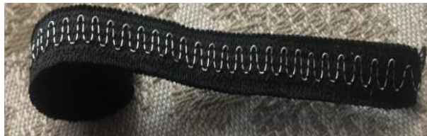
Figure 43: Elastic band with copper wire embedded.
