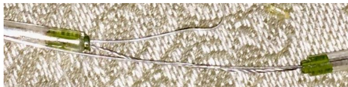
Figure 24: Detail of the series configuration between two microsprings.
