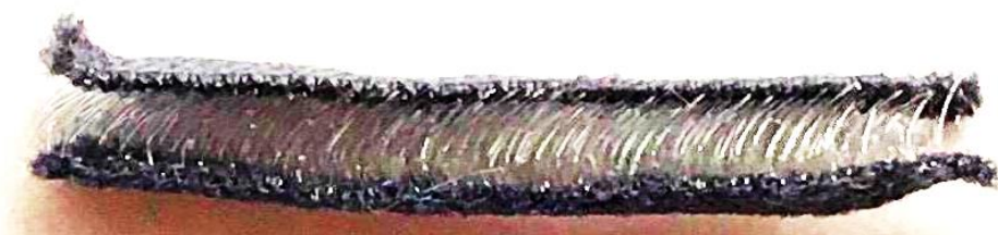
Figure 18: 4XD elastomeric structure. The micro elastomer filaments sandwiched between the two surfaces. This structure allows the fabric to move in the three directions with a certain elasticity.
