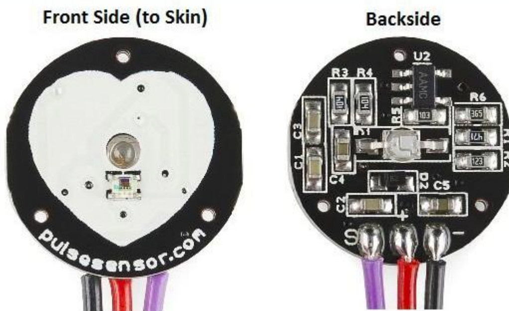
Figure 41: Pulse sensor amp device with 16mm diameter covered with vinyl stickers; front side (left image) and backside (right image) [45].
