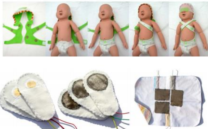
Figure 2: From top to bottom: Dressing process and test patches for textile electrodes [8].
