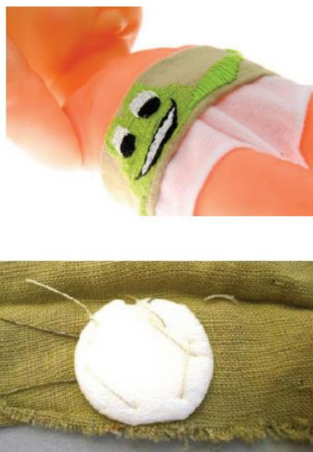
Figure 3 From top to bottom: The designed belt and the sensor isolation using foam[12] .
