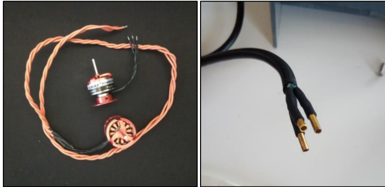
Figure 95. BLDC wires. Left: first version. Right: triphasic recycled cable.
