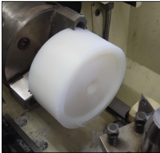
Figure 74. Operation of emptying of the back plug.
