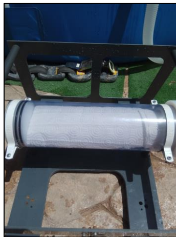
Figure 91. Tightness test with paper inside to verify if water goes in.
