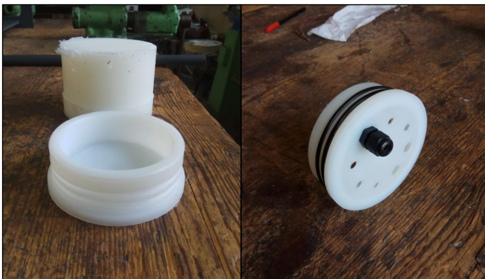
Figure 77. Back plug, before and after drilling holes.
