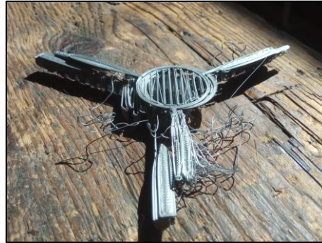
Figure 87. Defective propeller support.
