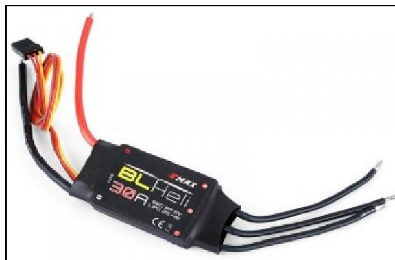
Figure 18. Electronic Speed controller, EMAX BLHeli 30A.
