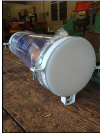
Figure 90. Test plug to check tightness.
