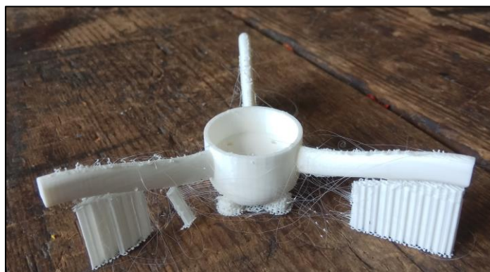
Figure 86. Propeller support after being printed.
