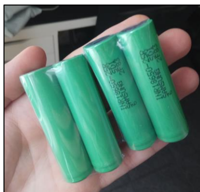
Figure AP 1. 18650 Samsung batteries
