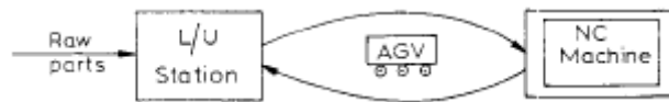
Figure 17. Case I: Simple manufacturing system composed by an AGV and a Machine
