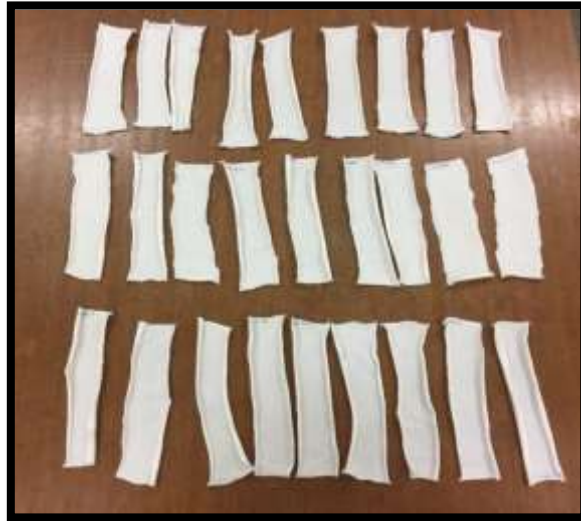
Figure 25. Samples needed to be left in the test room at the room condition.
