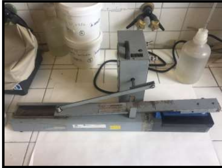
Figure 32. Crock meter used to conduct the rubbing test.
