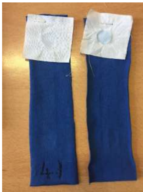
Figure 43. The products obtained for the rubbing fastness test (left) in dry state and (right) in wet state.
