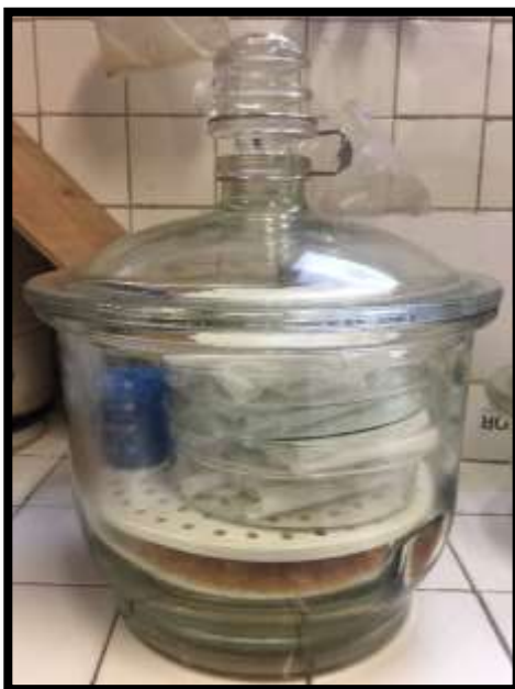
Figure 22. The dried samples were left in a desiccator before weighed to preserve the samples.
