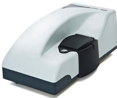
Figure 9 Zeta sizer nano zs 18
