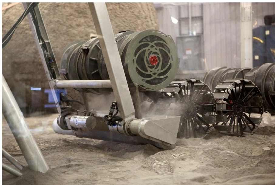
Figure 54: RASSOR demonstration of resource utilization (Kennedy Space Centre)
