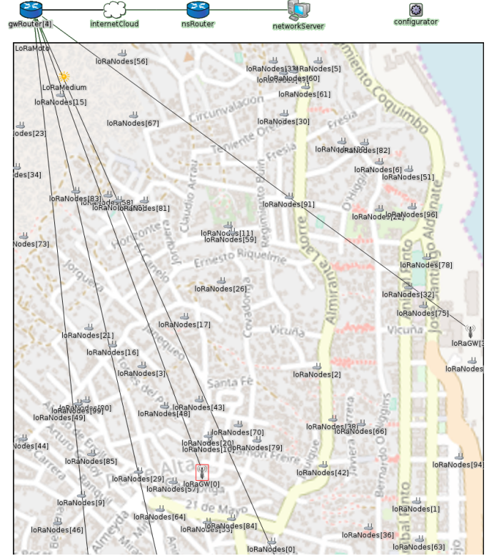
Figure 2. Screen capture of the OMNeT++ running the FLoRa framework, layered over the Coquimbo Peninsula OpenStreetMap imagery, showing the user nodes and gateways, and the remaining components on top.
