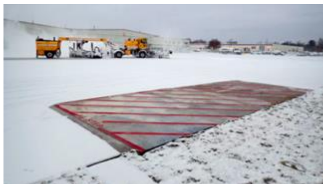
Figure 2.18 Thawing system test in a local airport [21]
