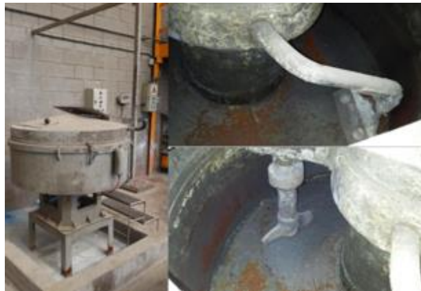
Figure 3.3 Kneading station and mixing rotating paddles
