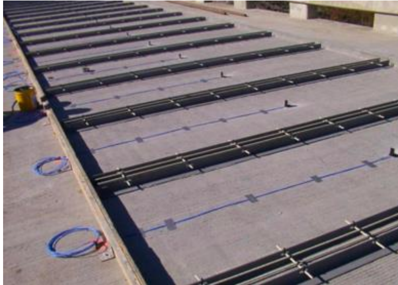
Figure 2.20 Iron angles electrodes and wiring disposal
