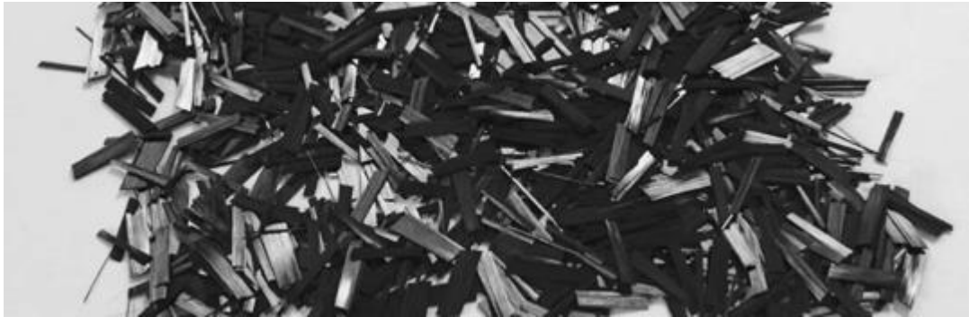
Figure 3.2 Carbisol™ CT6/12 chopped recycled carbon fibre (ELG Carbon Fibre LTD)
