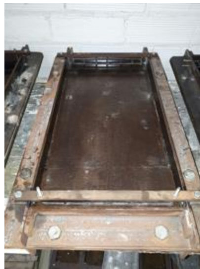
Figure 3.8 Slab mould of 300x600x40mm
