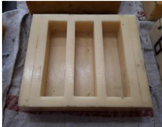
Figure 3.6 Three samples production mould of 40x40x160mm
