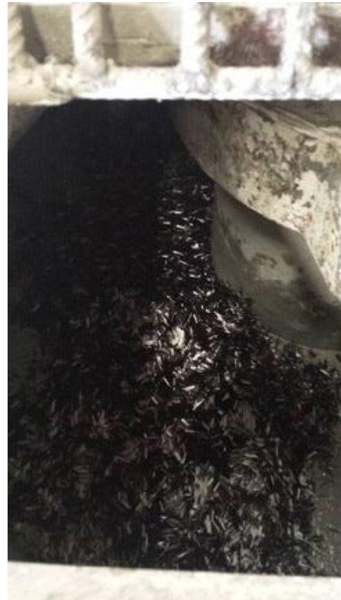
Figure 3.4 Addition of the recycled carbon fibres to the mix
