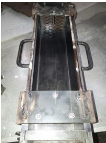
Figure 3.9 Beam mould of 10x10x400mm
