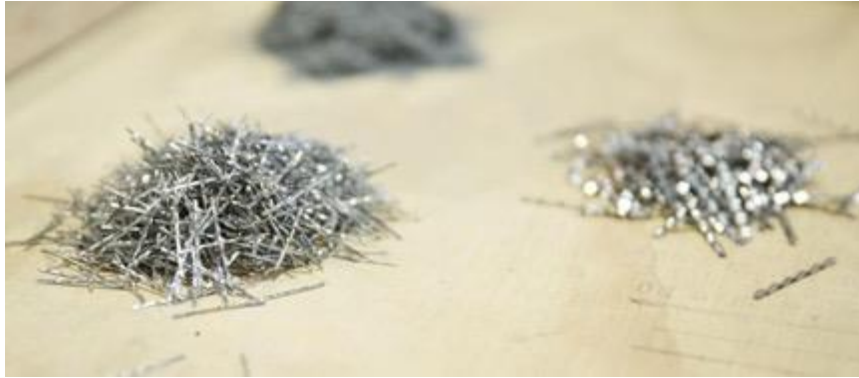
Figure 2.8 Special steel shavings for conductive concrete mix ( www.omaha.com )
