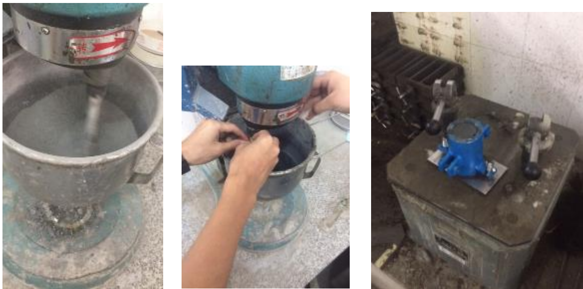
Figure 3-7 Mixing of powder (left); adding steel fibers (center); specimen after vibrating (right)
