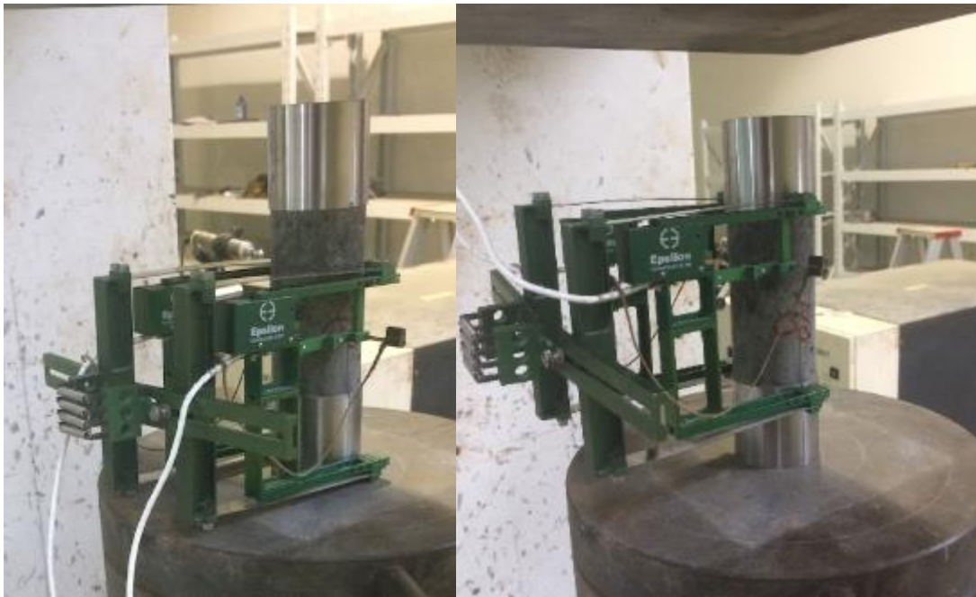
Figure 3-9 Test setup with the adapter cylinders
