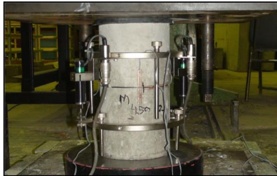
Figure 3-11 Example of LVDT placement [124]
