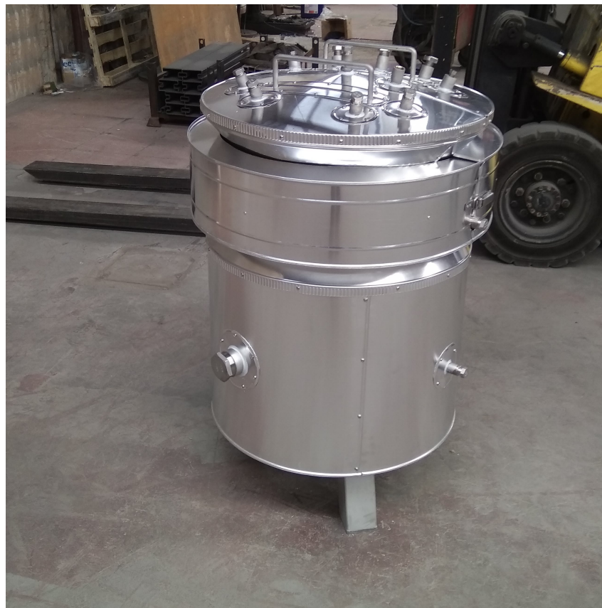
Figure 3.2: PEMFC's Oil tank.
