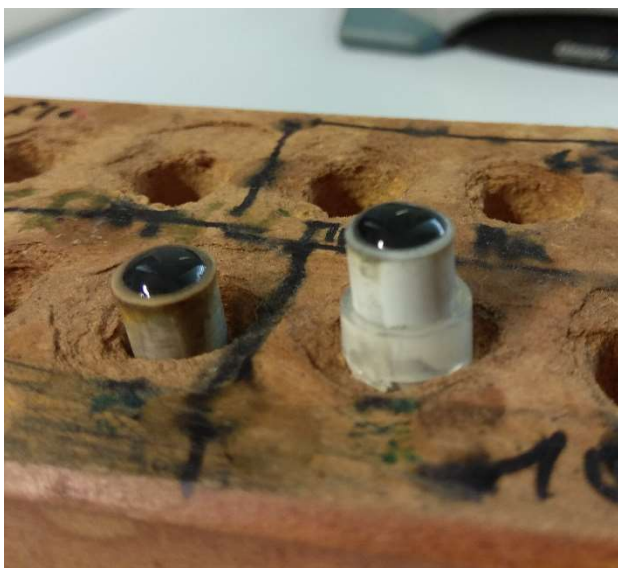
Figure 5.3 Electrode mixture deposition in conventional electrodes.
