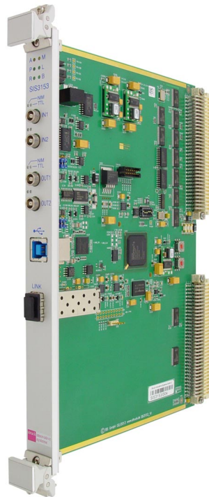
Figure 5.23: Photograph of the SiS3153 VME module from Struck, which in our setup is the ethernet to VME interface [229].
