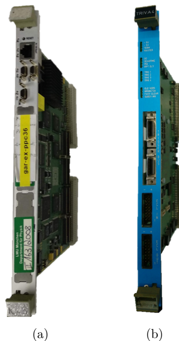
Figure 5.21: Photograph of the VME-based RIO-3 PowerPC frontend CPU [241] and the TRIVA 5 Trigger Unit [240].
