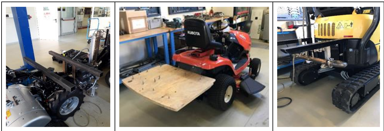
Figure 11. Mechanical works necessary to assembly the EFM. Detail of flexible pipe to connect the tail pipe.
