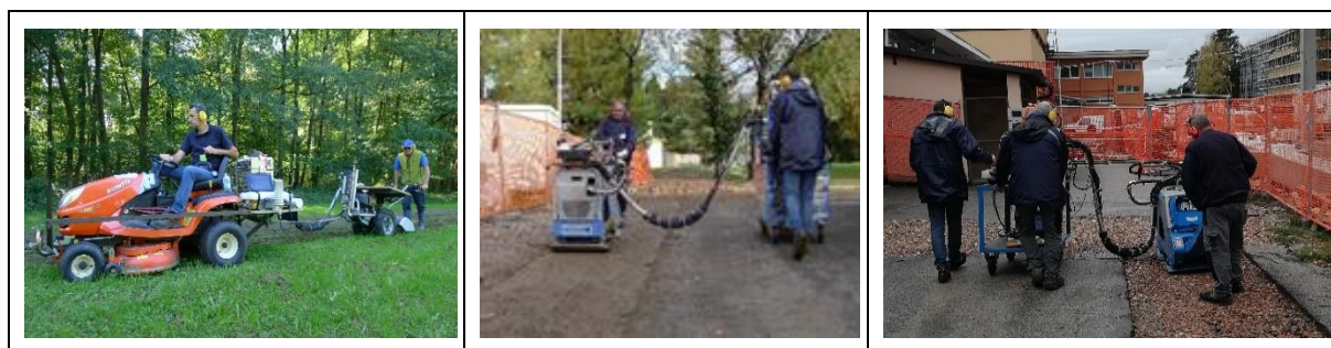
Figure 13. Use of a trolley or an additional vehicle to support the installation of the equipment (gas analyser, EFM, battery).
