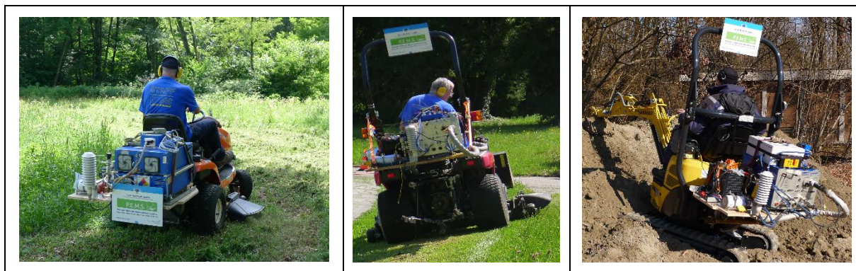
Figure 12. Machinery equipped with PEMS – Final Installation.
