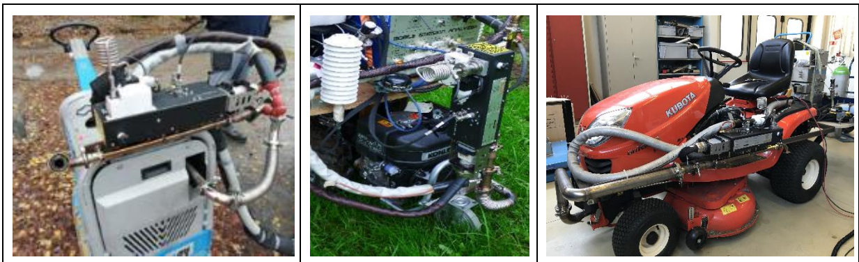
Figure 11. Mechanical works necessary to assembly the EFM. Detail of flexible pipe to connect the tail pipe.
