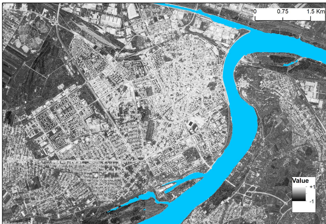
Figure 3. The output from the Association analysis - Evidence-based Normalized Differential Index in Novi Sad (Serbia). Water is shown with blue colour.
