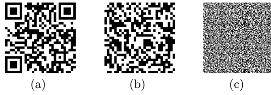
Fig. 5. Example of S , S_E and S_T (a) QR code containing secret message; (b) encrypted QR code; (c) result after Arnold transform.
