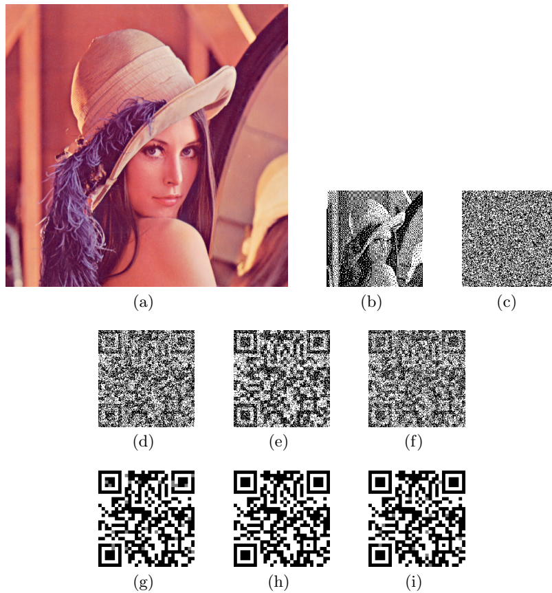
Fig. 6. Example results for the ‘lena’ image (a) input image; (b) dithered LL_2 sub-band; (c) visual depiction of the verification string; (d) S_R after JPEG compression; (e) S_R after noise; (f) S_R after blurring; (g) reconstructed QR code from Fig. 6(d); (h) reconstructed QR code from Fig. 6(e); (i) reconstructed QR code from Fig. 6(f).
