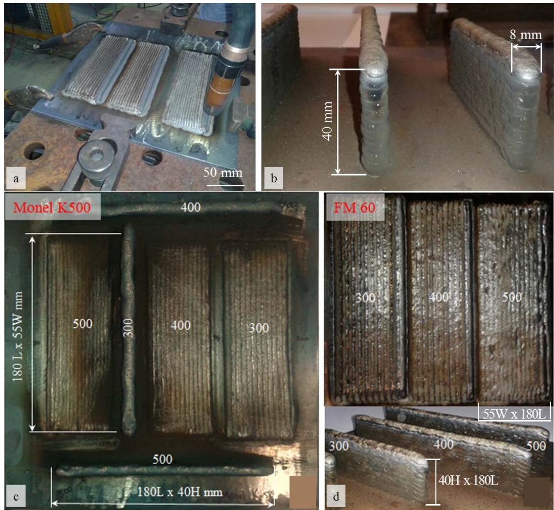
Figure 3.2 Wire arc additive manufacturing process: (a) deposition of multi-bead single-layer plates; (b) deposition of single-bead multi-layer walls; plates and walls produced at travel speeds of 300, 400, 500 mm/min with (c) Monel K500 and (d) FM60.
