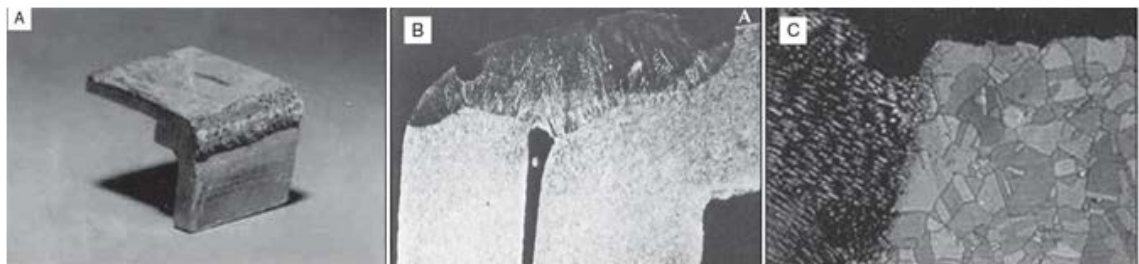
Figure 2.35. (a) A corner welded of Monel 400, (b) the corner cross section, (c) localised corrosion at the fusion boundary [74].
