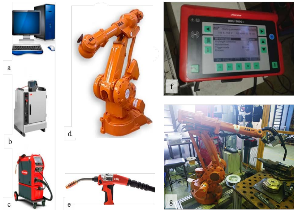
Figure 3.1. Schematic diagrams of the WAAM system: (a) computer, (b) robot controller, (c) welder, (d) ABB 1400 robot, (e) CMT welding torch, (f) control panel, (g) set up of the robotic CMT process.
