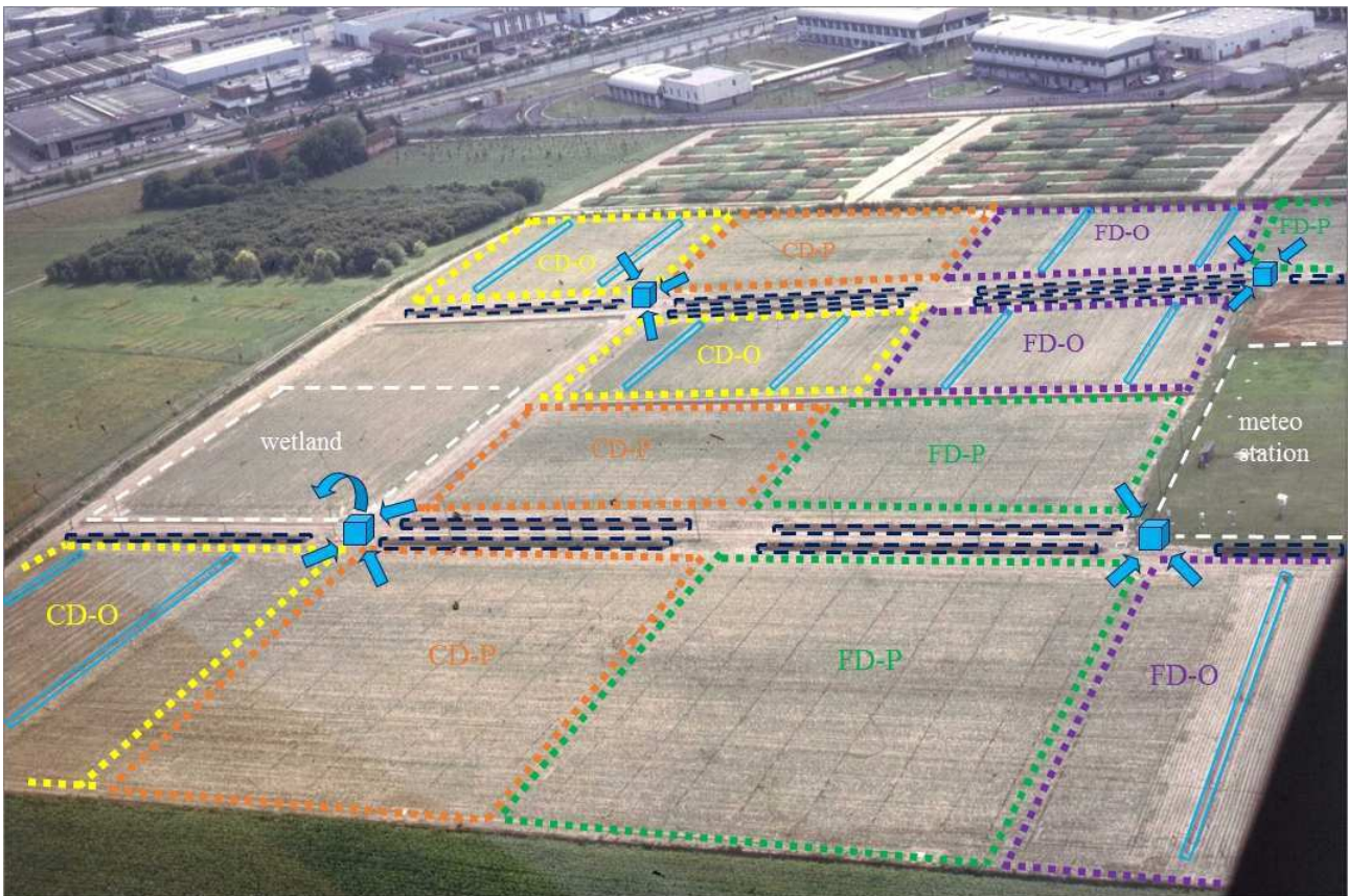
Fig. 2.2. Aerial view of the experimental fields. CD-O: controlled drainage with open ditches (yellow); CD-P: controlled drainage with subsurface pipes (orange); FD-O: free drainage with open ditches (violet); FD-P: free drainage with subsurface pipes (green). In light blue: open ditches of CD-O and FD-O, and sumps (cubes) that collect outflow water from each plot. In dark blue: delivery ditch for each plot. In white: surface flow constructed wetland and meteorological station.
