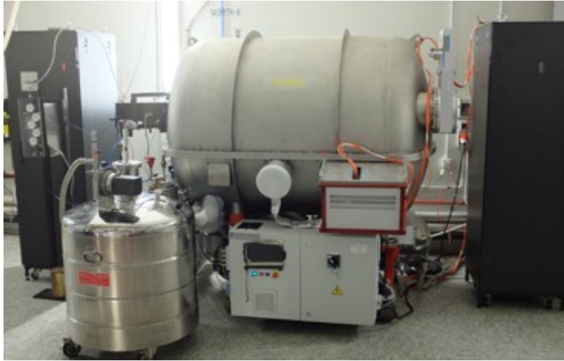
Figure 2.2: GIANO vacuum vessel, fiber agitator, LN2 tank and the electronics in the Nasmyth A of TNG (Claudi et al., 2016)
