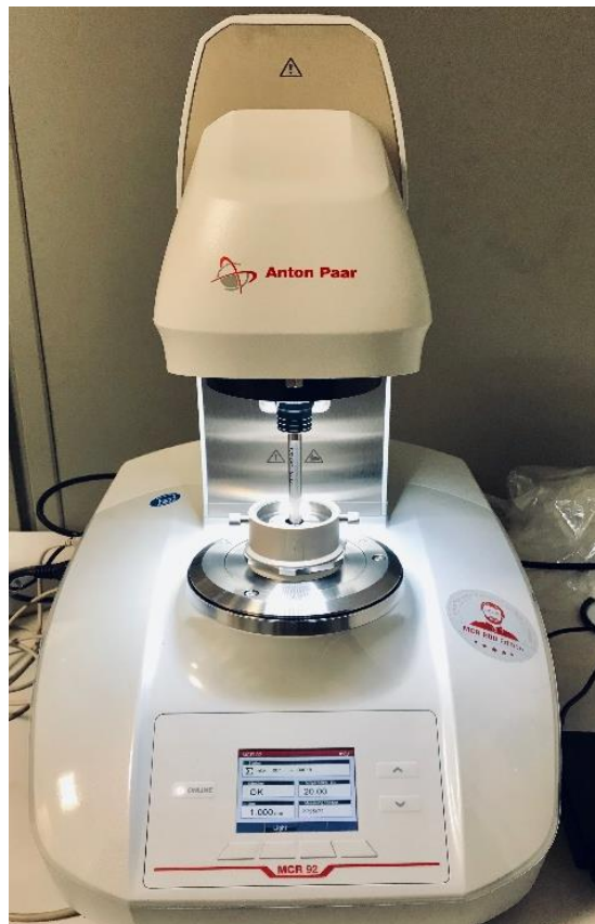
Figure 8. Rotational rheometer MCR 92, Anton Paar.
