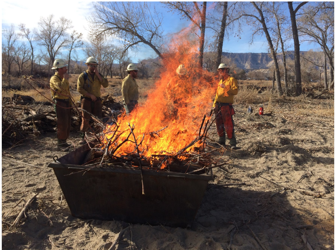
Figure 1. Metal biochar kiln processing feedstock in Utah.
