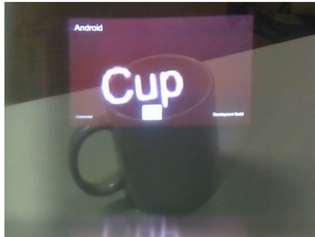
FIGURE 6.14: View through Glass display of a cup overlaid with an AR annotation.
